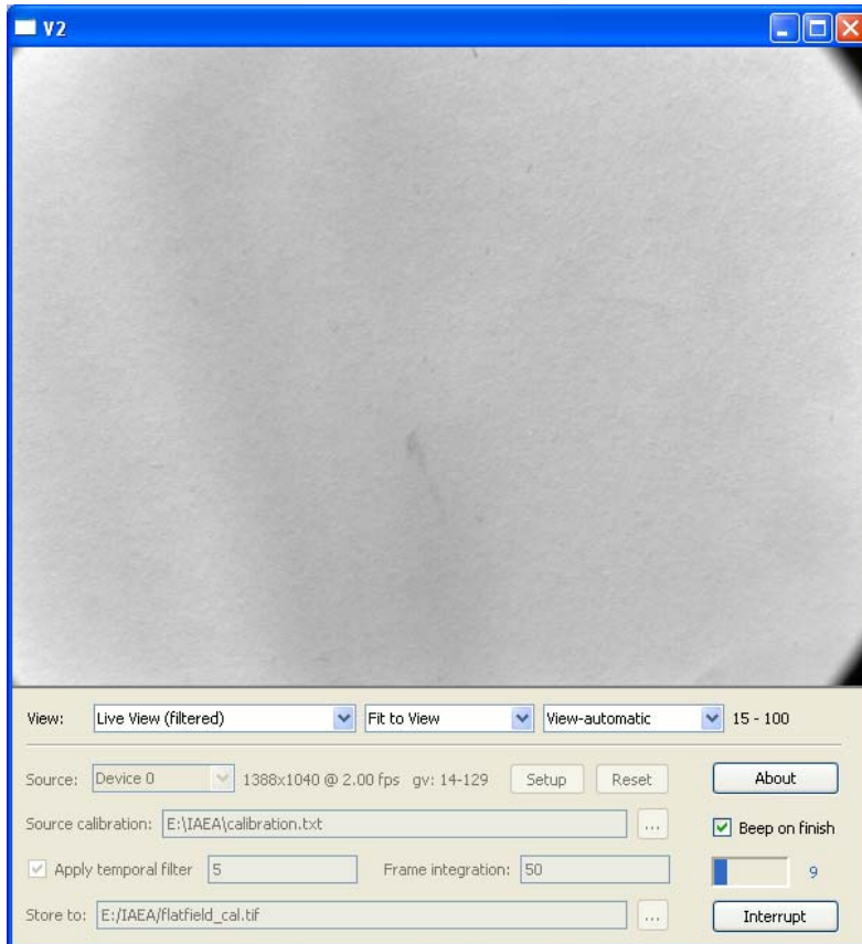
Fig. 7: Example of ongoing integration with V2 (9 frames of 50 are already done) using all features including calibration. The acquired gray values of a single frame are between 14 and 129, so no clipping is shown and the source calibration should work also. The computer load by the applied temporal filtering of 5 frames and image integration decreases the frame rate from 5 fps to 2 fps. So an overall exposure time of 50 \times 0.2\text{s} = 10\text{s} is integrated, but the time needed for this integration is 50 \times 0.5\text{s} = 25\text{s} ! So a faster computer will save some overhead exposure time.
